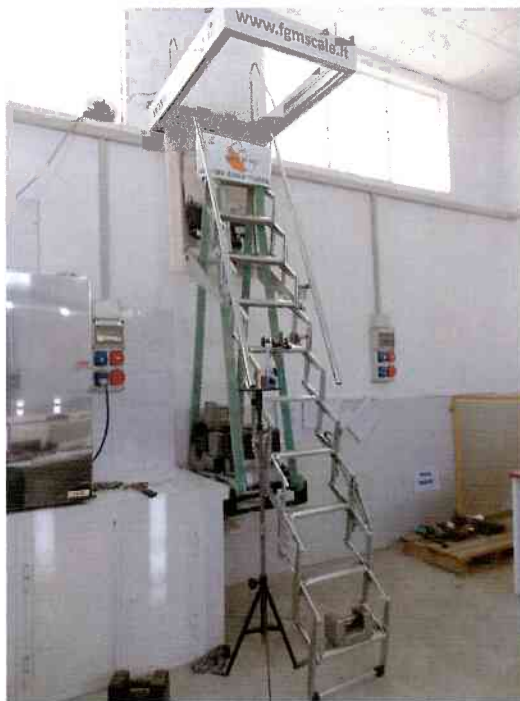
Picture 1: static load test – first step
