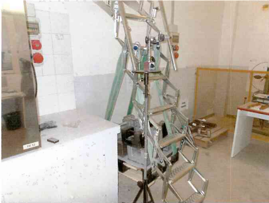
Picture 3: static load test – middle step of the ramp, specific dial gauge
